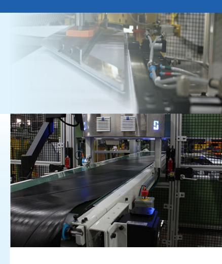
The latest Steelastic extruded belt systems make it possible to produce passenger, truck / bus and specialty tires without calendering and off-line cutting. Closed-loop automation minimizes operator involvement through the use of the very latest measurement technologies and closed-loop control.
