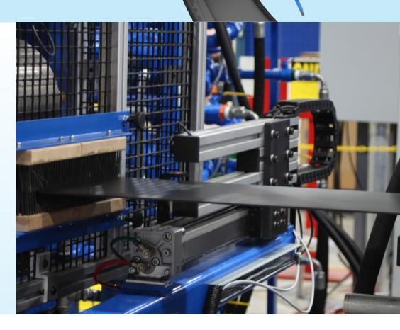
Mounted between the die head exit and cooling drum entrance, this system uses a single-point laser measurement system that continuously traverses back and forth across the extruded strip to verify the average gauge.
