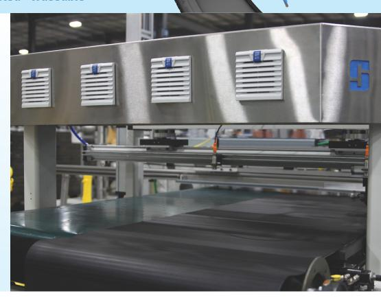
The assurance vision inspection system uses 3D laser vision technology to identify and report defects in real-time during the production of radial belt and body ply materials to guarantee a defective product never makes it to the tire building process. We remain committed to delivering the best quality system upgrades to meet your most demanding production and quality requirements.
